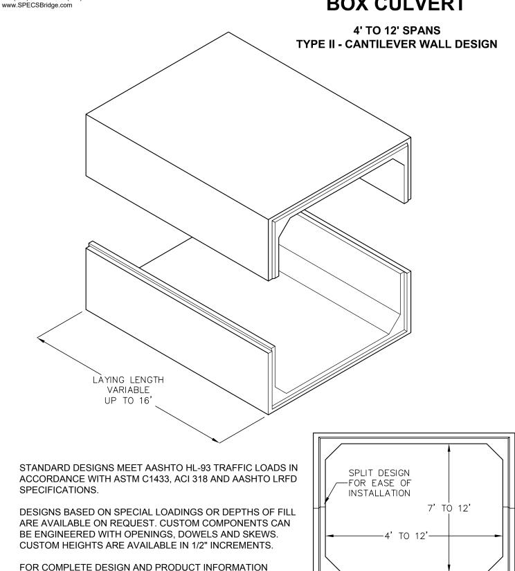
ENDS CAN BE SKEWED TO ALLOW FOR CURVES IN CULVERT RUN -- NO NEED FOR SECONDARY FILLLER POUR.
