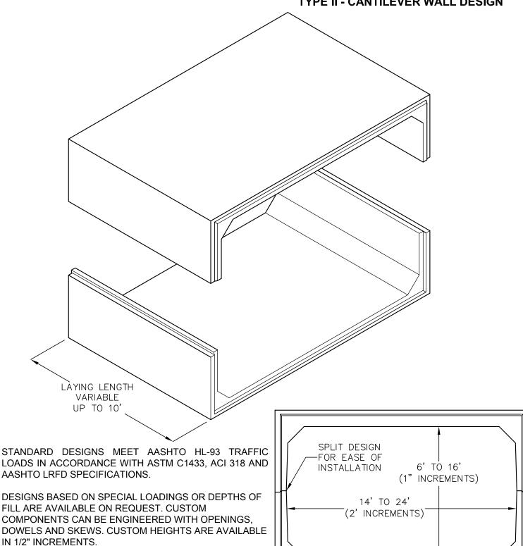
ENDS CAN BE SKEWED TO ALLOW FOR CURVES IN CULVERT RUN -- NO NEED FOR SECONDARY FILLLER POUR.
